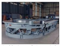
Receiving Conveyor for Desprue, Sorting and Grinding (oval conveyor)
