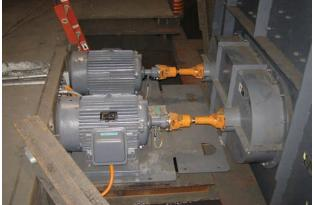
The original shakeout system used wooden rails (above) to minimize damage to flasks during cleaning; the drive system on the new Delta-Phase® shakeout (below).
