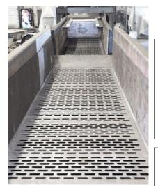
The new machines have 1.5-in. thick steel decks stiffened to withstand impacts from 1,600-lb. steel castings, and cut with back-drafted slots to maximize sand removal and minimize product jamming.
